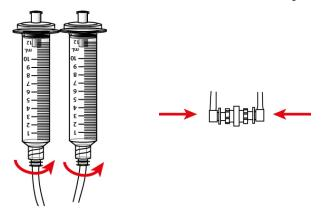
Check the tightness of the connections!
